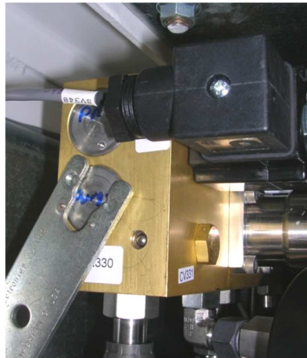
Figure 55 – Removing the Orifice Cap with Spanner Wrench
