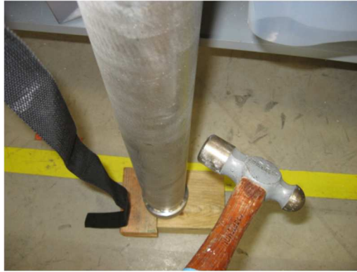
Figure 50 - Desiccant at the Top of the Cylinder and Tapping the Cylinder
